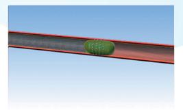
A propellant bypass along/through the pig body provides the discharge of the deposits to be removed, in order to prevent a blockage.
